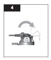
• Pinch wire form to release the safety cap.
