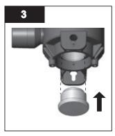
Insert the sleeve removal tool at the bottom of the sleeve.
