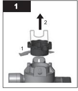
Remove the sleeve bolt from top of the sleeve assembly.
