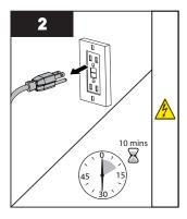
Disconnect main power source and allow the unit to cool for 10 minutes.
