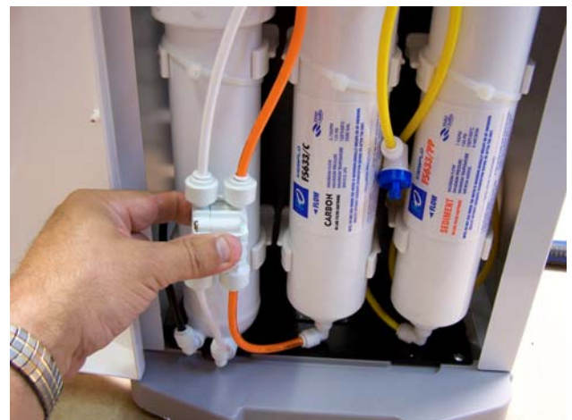
RO filter set showing autovalve. The autovalve automatically turns off the water flow when the tanks are full
